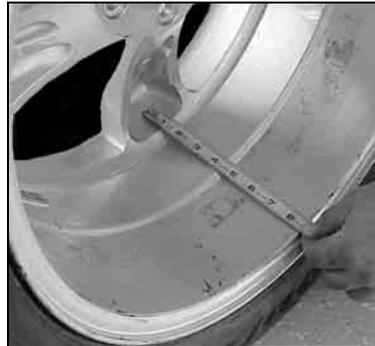
Measure the weight plane diameter manually, using caliper.
