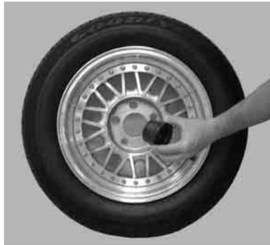
**NOTE:** If the basic cone and adaptors do not fit the wheel, additional centering adaptors will be necessary. A wheel that cannot be properly centered, cannot be properly balanced. All balancers require additional centering adaptors to properly center certain types of wheels. For additional information, refer to Form 3203T for optional accessories.
