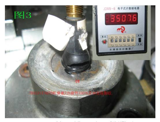
4. TR414(28%EPDM08070202)臭氧 72h 疲劳 59399 次 1#3#嘴体断裂图片 after flex testing 59,399 times, 28%EPDM No.1# and No.3# tire valve was cracked
