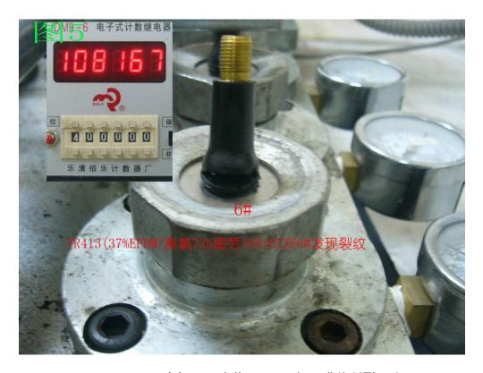
6. . TR413(37%EPDM211-14)臭氧 72h 疲劳 163080 次 5#嘴体断裂图片 after flex testing 163,080 times, 37%EPDM No.5# tire valve was cracked
