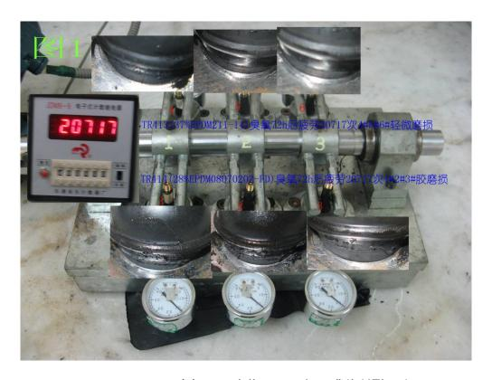
2. TR414(28%EPDM08070202)臭氧 72h 疲劳 31429 次 2#嘴体断裂图片 after flex testing 31,429 times 28%EPDM No.2# rubber were cracked
