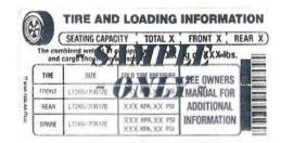
Tire pressure should be checked and set with cold tires before the vehicle is driven. It is necessary to adjust air pressure in tires periodically. Tire pressure changes with outside air temperature, and can lose approximately one pound per square inch (psi) of air pressure per month.
