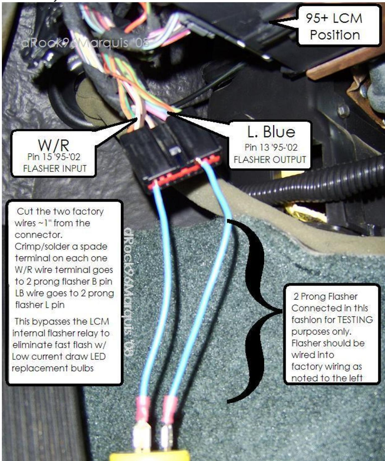
As mentioned in that picture, you need to cut the wiring before the LCM
