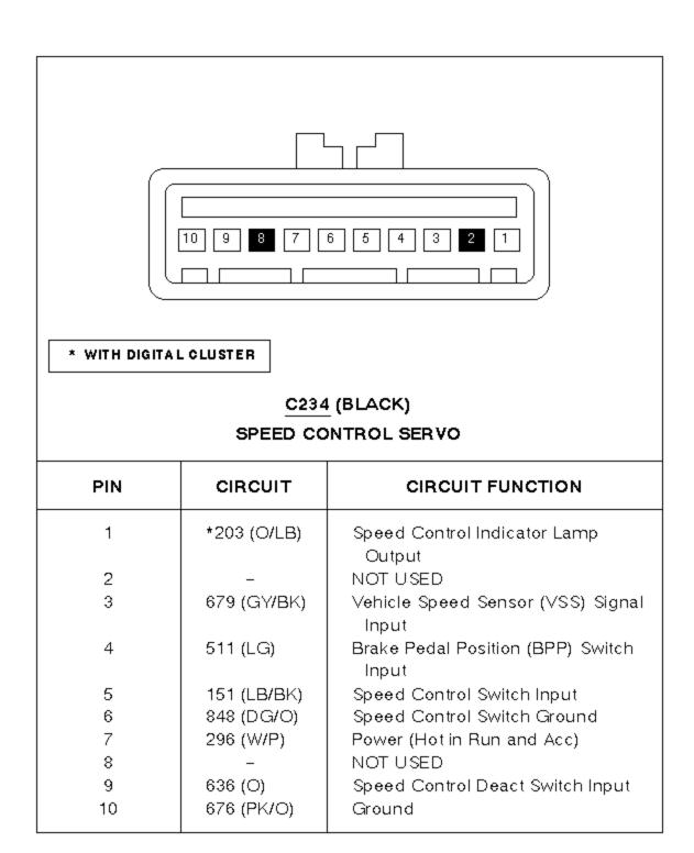
Note: For vehicles without speed control, a cap containing a shorting bar is placed over the 10-pin servo connector. The shorting bar connects pins 6 and 10, providing a ground path for the steering wheel mounted horn switches. If this shorting bar is not present, the horn will not function. The part number for this item is F3TZ-14A666-A
