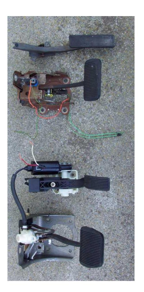
And here's a closeup of the speed control deac switches from a 98' crown victoria and a 01' grand marquis
