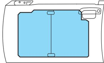
The above illustration is an outside view of the left front door. The shaded area represents the area covered by the ballistic door panel.
