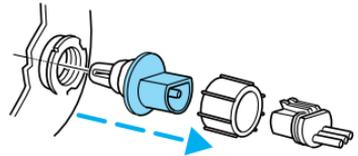
2. Install the bulb retaining ring over the plastic base until it contacts the rear of the socket by rotating it clockwise until you feel a "stop."
