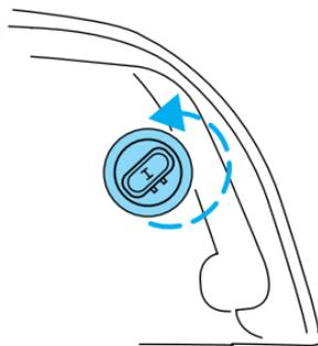
6. Carefully pull bulb straight out of the socket and push in the new bulb.
