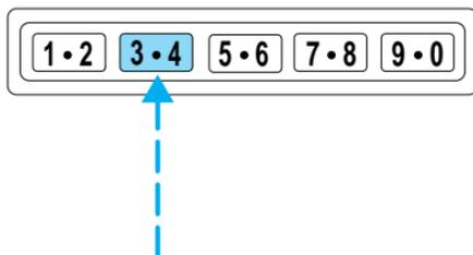
To release the trunk, enter the factory-set code or personal code (driver door unlocks) and press 5/6 within 5 seconds.
