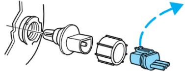
5. Remove the bulb retaining ring by rotating it counterclockwise (when viewed from the rear) about 1/8 turn to free it from the bulb socket, and slide the ring off the plastic base. Keep the ring to retain the new bulb.
