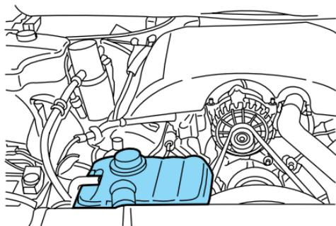
If the engine coolant has not been checked at the above recommended interval, the engine coolant reservoir may become empty. If this occurs, add engine coolant to the reservoir. For more information on engine coolant maintenance, refer to *Adding engine coolant* in this chapter.
