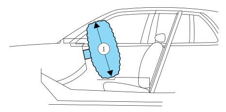
Figure 2  $1.\ 650\ \mathrm{mm}\ (25.5\ \mathrm{inches}).\ \mathrm{Cross}\ \mathrm{section}\ \mathrm{through}\ \mathrm{center}\ \mathrm{of}\ \mathrm{vehicle}$  (passenger side shown)
