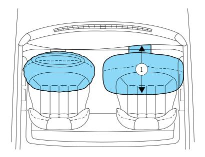
Figure 3  $\,$  1. 580 mm (23 inches). Front passenger compartment
