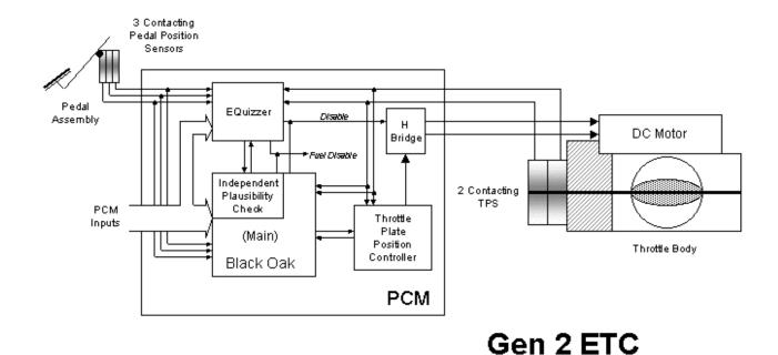
Because safety is a major concern with ETC systems, a complex safety monitor strategy (hardware and software) was developed. The monitor system is distributed across two processors: the main powertrain control processor and a monitoring processor called an Enhanced-Quizzer (E-Quizzer) processor.
