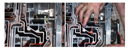
2. Install Valve Body. Torque the bolts to 10-12lbs. starting from the center outward. Still use your judgment and don't strip the threads. Install the retaining clip for the Transmission Pressure Solenoid.
