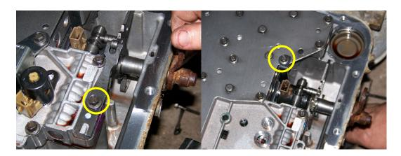
3. Loosen the rest bolts on the Valve Body. Just loosen the 10mm Bolts on the 98 Transmission. Just the bolts with the washers. You do not have to remove the plate. Just remove the valve body in one piece. Pull the plate off of the 94 Valve body.
