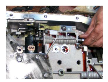
4. Install Shift Solenoids and TCC Solenoid. Don't forget the install the Grounding Clip for the TCC from the 94.
