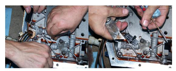
6. Now plug all the wires back in Install filter. Clean you pan and gasket. And install
