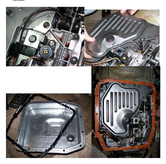
7. Torque your pan bolts flip the transmission over. Install the MLPS and the 94 Exterior Harness. Make sure you line up the MLPS properly. Switch out the Speed Sensor. PUT IT BACK IN YOUR CAR.
