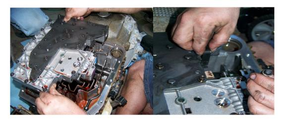
3. Install the Gear Selector Tensioner. Make sure the Gear Selector Valve is in the correct slot.
