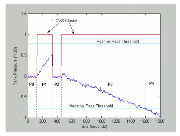
P0 = Phase 0, Stabilization Phase – With CVS open, Tank Pressure is allowed to stabilize. A fuel volatility test is performed and FTPT offset correction is learned if volatility test passes.
