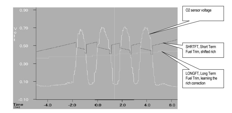
As components continue to change beyond normal limits or if a malfunction occurs, the long-term fuel trim values will reach a calibratable rich or lean limit where the adaptive fuel strategy is no longer allowed to compensate for additional fuel system changes. Long term fuel trim corrections at their limits, in conjunction with a calibratable deviation in short term fuel trim, indicate a rich or lean fuel system malfunction.
