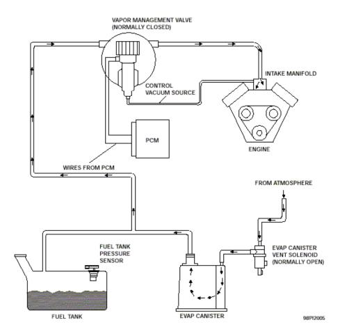
The evap system integrity test is done under conditions that minimize vapor generation and fuel tank pressure changes due to fuel slosh since these could result in false MIL illumination. The check is run after a 6 hour cold engine soak (engine-off timer), during steady highway speeds at ambient air temperatures (inferred by IAT) between 40 and 100  $^{\circ}$ F.
