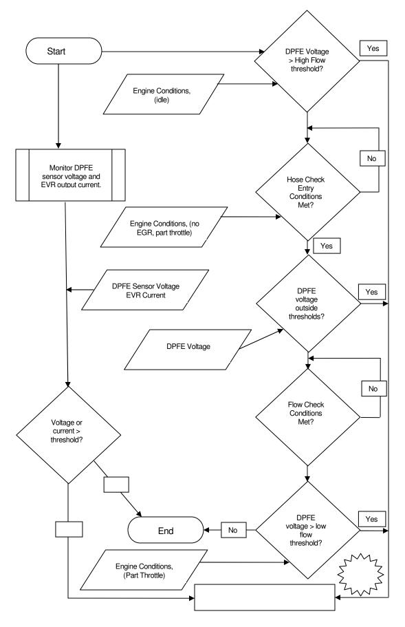
The Delta Pressure Feedback EGR Monitor is a series of electrical tests and functional tests that monitor various aspects of EGR system operation.
