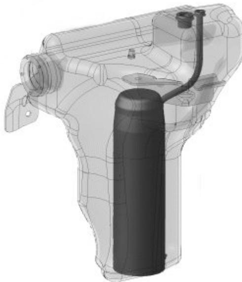
**Figure 4. Diagram of the left-hand bottle showing gas generator integrated inside (distribution system not shown).**
