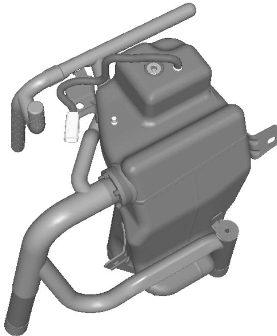
**Figure 5: Right Hand Suppressor and Distribution System.**
