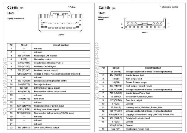
(05+ LCM pinouts are a little different but the wiring colors remained the same for these two functions)
