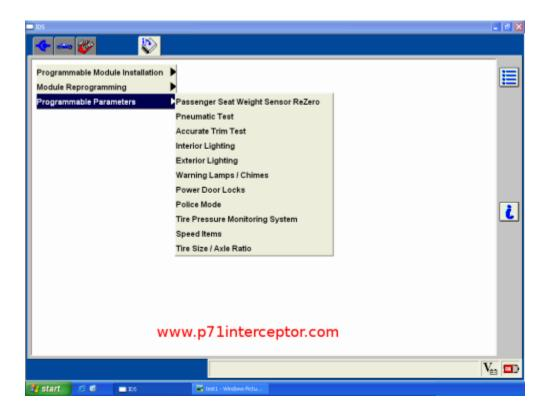
This section of the ids program is used after installing new passenger seat weight sensor components or after installing a different passenger seat assembly. If this procedure is not completed after those tasks, the airbag system might not work properly and the airbag warning light on the instrument cluster might be illuminated.
