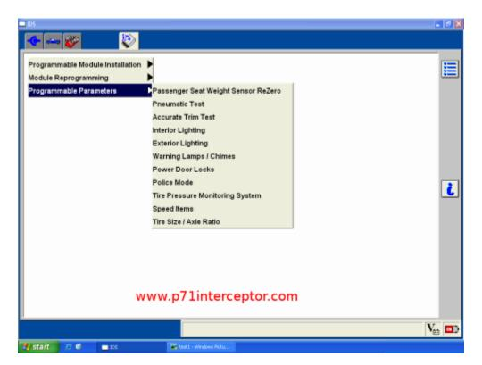
Do not enable the Daytime Running Lamps feature unless you have the drl module present under the hood. Canadian vehicles usually have this module factory installed. Vehicles for the United States market usually don't.
