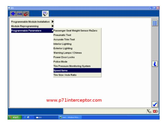
And now speed control is present. If we have a new steering wheel with the cruise switches already installed, we should be able to utilize cruise control now.
