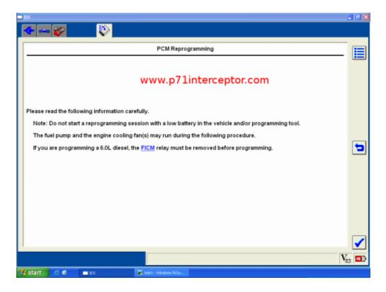
Turn the ignition key to the run position, but do not start the engine
