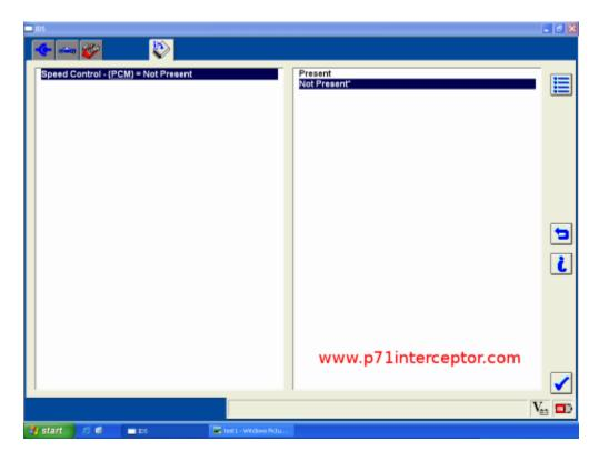
This particular police cruiser didn't have factory installed cruise control. So we're going to enable it by clicking on "Present"
