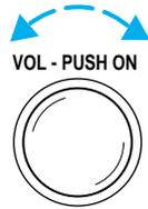
If the volume is set above a certain level and the ignition is turned off, the volume will come back on at a “nominal” listening level when the ignition switch is turned back on.
